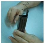
3. Holding the mag spacer in place, insert the follower and mag spring into the mag tube and tight against the feed lips.
