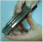
2. Insert the mag spacer all the way to the top of the mag tube with radiused edge facing the back of the mag tube.
