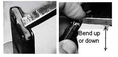
Hold the tool firmly against the lip with the index finger of the hand holding the clip while rotating the tool up or down with the other hand. Bending the lips in (rotating the tool end upward in the picture) will lower the feed angle and opening the lips (rotating the tool end downward) will raise the feed angle.
