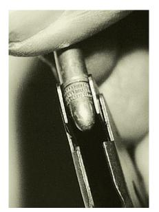
Check that the bullet itself slips freely between the front lips. The bullet shouldn't stick, but there shouldn't be excessive space between the bullet and lips either. To check for too much space, try to wiggle the case back and forth. If there's play, tighten the lips. Try to strip a round out of the magazine. The round shouldn't stick or bind.
