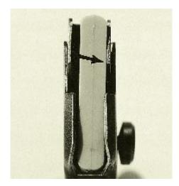
Gauge the inside of the rear of the front lips of the magazine The dimension should be 0.230 inch. Adjust the rear of the front lips of the magazine as needed. Keep the lips parallel.
