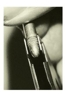
Check that the bullet itself slips freely between the front lips. The bullet shouldn't stick, but there shouldn't be excessive space between the bullet and lips either. To check for too much space, try to wiggle the case back and forth. If there's play, tighten the lips.
