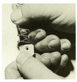
Reassemble the magazine properly. The follower fits into the end of the spring that has only a half coil. The spring should slip easily over the follower.
