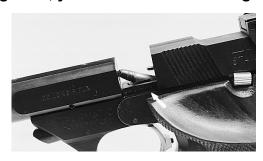
Clean and lightly oil the top of the frame where the slide moves (arrow). This corrects many return-to-battery and cycling problems instantly.
