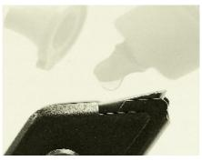
Oil and work the magazine spring. Small amounts of bluing salts inside the magazine can prevent the ammo from advancing smoothly. We recommend Marvel Mystery Oil because it neutralizes any remaining salts left on the metal. Often, the shooter feels the presence of these salts inside the magazine shaft as rough spots. Working the spring up and down the magazine will point to problem areas, and the oil will break them up. Remove excess oil as necessary once you've finished
